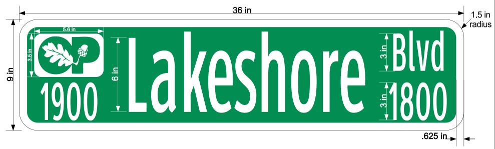
Street signs shall be manufactured with 3M<sup>™</sup> High Intensity Prismatic Sheeting and 3M<sup>™</sup> Green ElectroCut<sup>™</sup> Overlay Lettering shall be 6" mixed-case ClearviewHwy<sup>®</sup> font.
